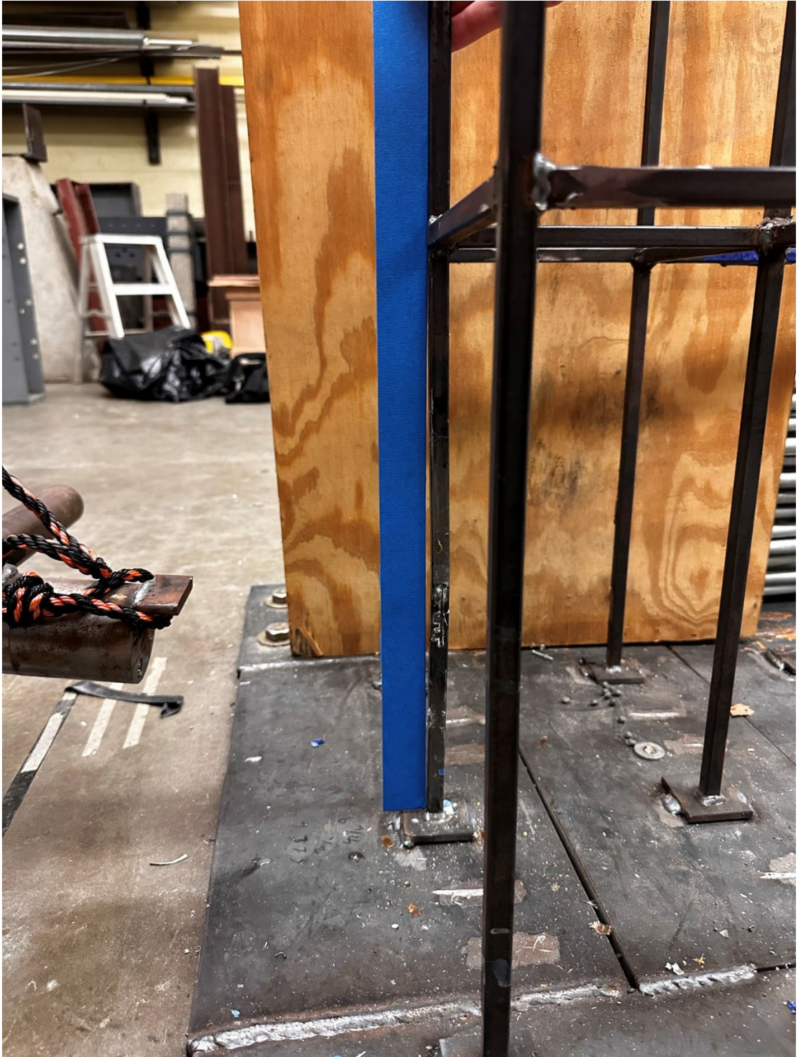
Figure 92. Ground-level column of model frame after impact with q = 18 in.
