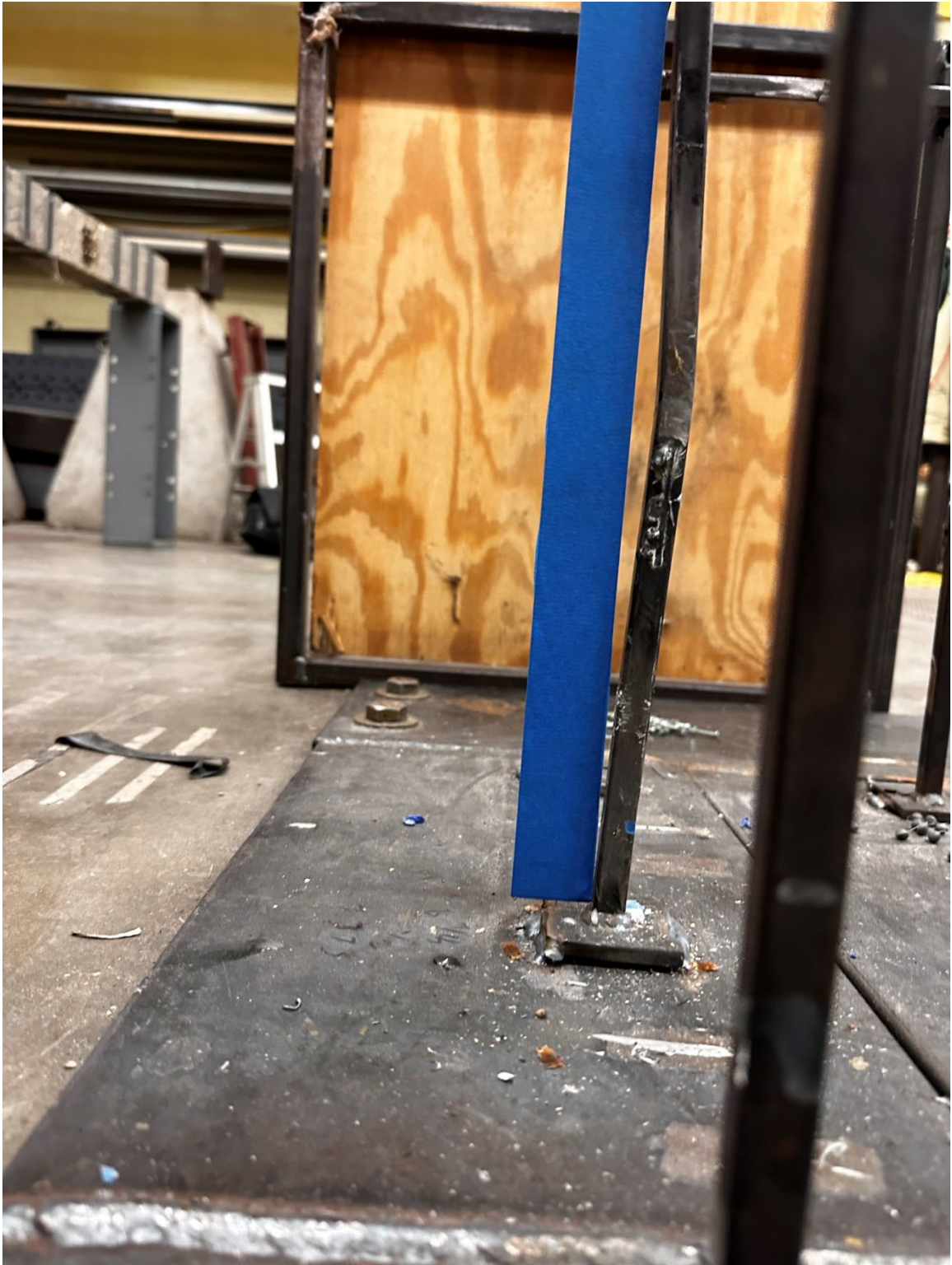
Figure 97. Ground-level column deformation of model impacted with q = 25 in.
