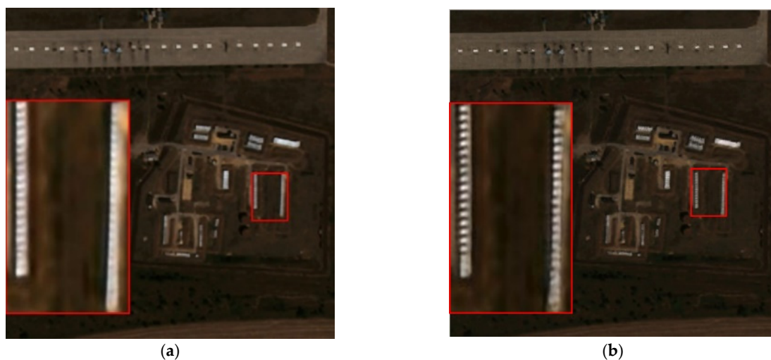
Figure 9. Visual comparison for high-frequency details of images fused by the U-Net (a) and HRNet backbones (b). For this experiment we choose Experiment 1 with 6\times . The large red box contains the zoomed-in region in the small box.
