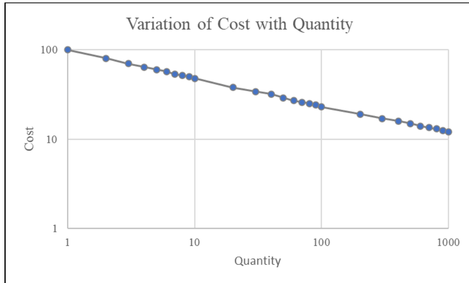
Figure 3: Eighty Percent Labor Curve – Data Extrapolated from Wright (1936)
