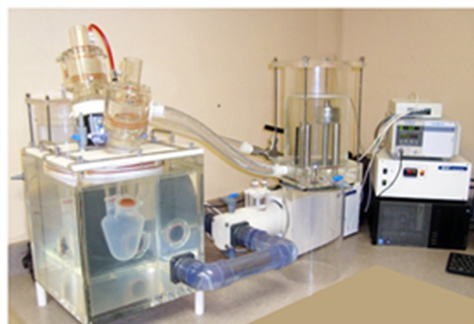
Figure 7. Left – DU pulse duplicator system; Right – valve prepped for testing in a washer to be mounted in the pulse duplicator.
