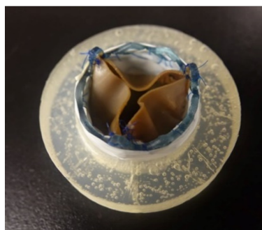
Figure 7. Left – DU pulse duplicator system; Right – valve prepped for testing in a washer to be mounted in the pulse duplicator.
