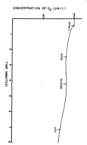
Figure 9. Clark electrode trace of oxygen uptake by Phycomyces blakesleeanus spores showing effect of glucose (10 mg/ml), acetate (0.72 mg/ml), malonate (0.017M), potassium cyanide (KCN) (0.001M), sodium azide (0.001M). Reaction mixture prepared in phosphate buffer (pH 5, 0.067M), spores (5.3 mg dry weight) in a total volume of 3 ml. Chemicals were added dissolved in 0.1 ml buffer except for glucose which was added dry.
