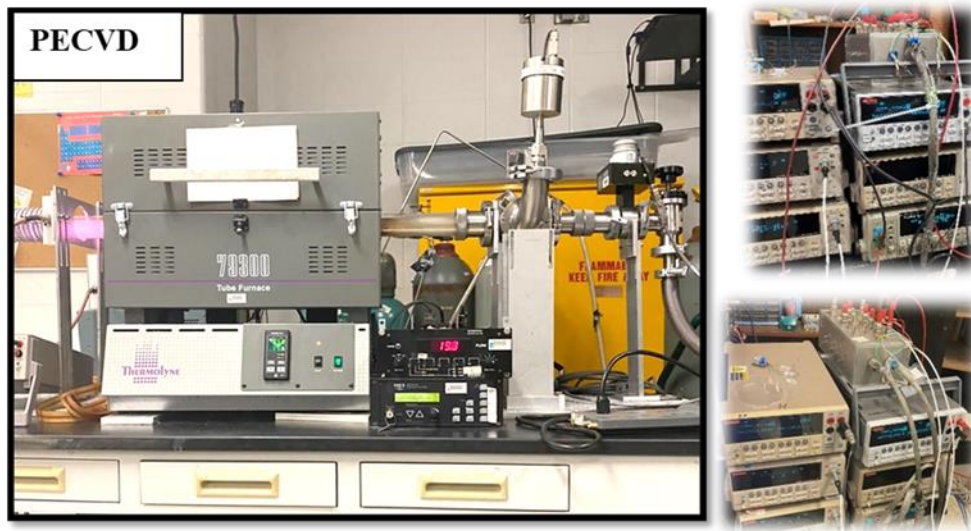
Figure 34: (a) Synthesis of in-situ Nitrogen doping of Graphene (b) thermopower/resistance measurement setup.
