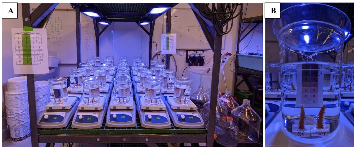
**Figure 2.** (A) Static renewal exposure system using 1.5L glass beakers with Teflon-coated magnetic stir bars on stir plates. (B) Beakers were covered with watch glasses to prevent evaporation.
