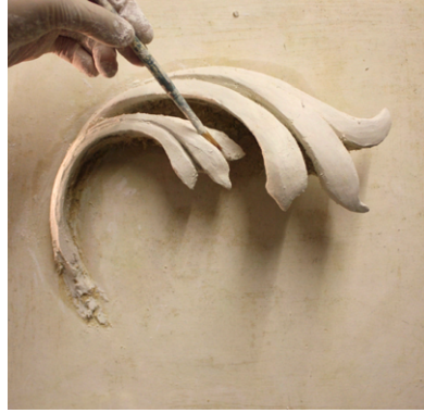
Figure 9.23: Lime-plaster modelling demonstration.
