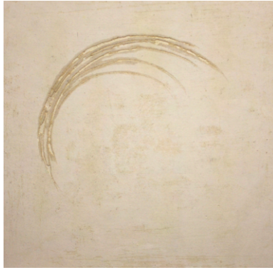
Figure 9.9: Lime-plaster modelling demonstration: a scratched line.
