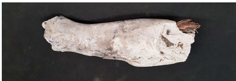
Figure 1.29: Lower-leg fragment, revealing the use of bundles of straw or reeds held together by drawn wire.
