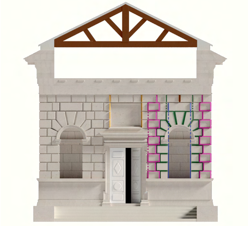
Figure 7.17: Printing House, Trinity College Dublin, inner wall of portico, alignments of vertical channels of rustication.
