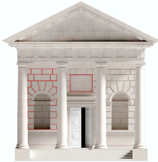
Figure 7.15: Printing House, Trinity College Dublin, elevation showing relationship of columns to inner wall of portico.
