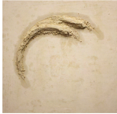
Figure 9.11: Lime-plaster modelling demonstration.
