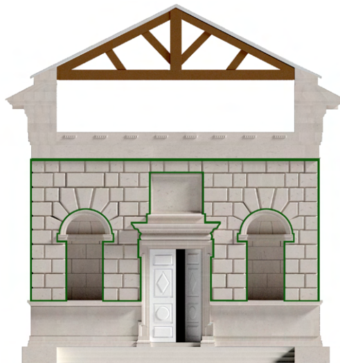
Figure 7.14: Printing House, Trinity College Dublin, with rusticated field outlined.
