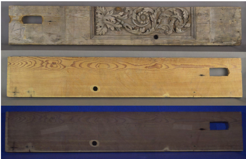
Figure 2.29: Section of a pine newel post cut off during the 1956/57 installation of the Cassiobury staircase. The front of this fragment shows the whitish haze, dust and grime (top), while the back reveals the natural colour of the wood (centre). The edges show the depth the stripping chemicals penetrated into the wood (up to half an inch [15 mm]), which is especially noticeable in UV light (bottom). Note that the more recently cut edges show no penetration.
