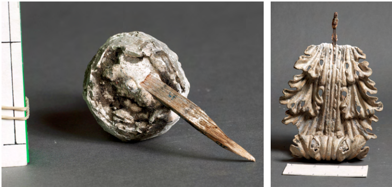
Figure 3.20: (a) Peach plaster fragment, showing timber armature, No. 129 St Stephen's Green, Dublin; (b) acanthus leaf, showing nail armature, entrance hall ceiling rose, South Frederick Street, Dublin.
