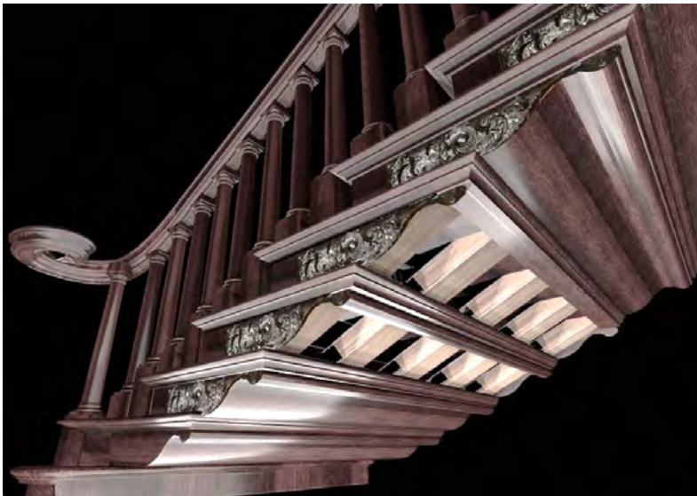
Figure 11.19: Structure of the staircase at No. 85 St Stephen's Green, Dublin.
