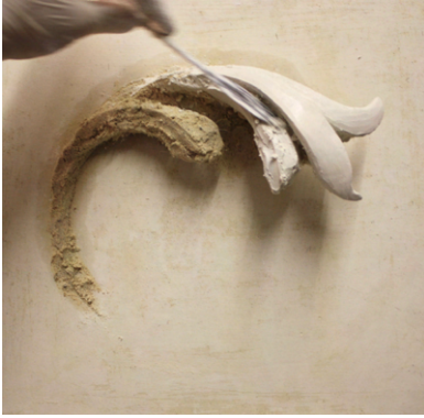
Figure 9.22: Lime-plaster modelling demonstration.
