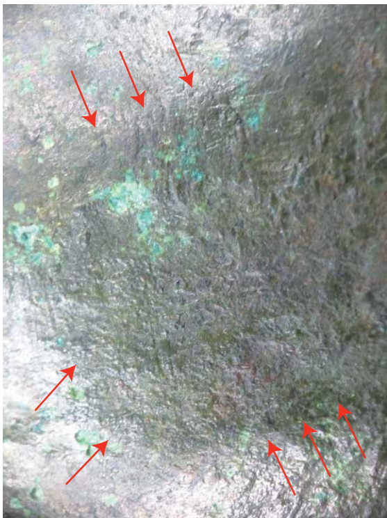
Fig. 21. Detailed images of the flat axe from Neuenkirchen: 1.-2. Indicated marginal ridges; 3.-4. Raised material on the fracture surface; 5.-6. Dents on the sides of the blade (1.-5. author's images, 60x magnification).
