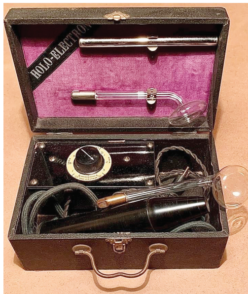
Figure 6. Holo-Electron violet rays apparatus complete with glass electrodes, bakelite handle, and voltage control. About 1920. Photograph by the author.
