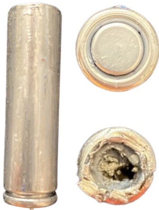
FIGURE 1. Representative cylindrical AA battery with negative electrode removed and visible internal contents.
