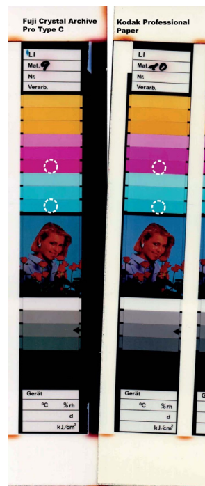
Figure A1. Chromogenic test strips used for measuring reflection density spectra: a Kodak Professional Paper and a Fuji Crystal Archive Pro Type C. The white dotted circles indicate the locations being measured. Source: Hofmann-Sievert, R. 'Contemporary Silver Halide Colour Photography', workshop demonstration, University of Amsterdam, 4 December 2019.
