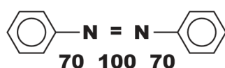
Figure 2. Schematic of azo dye with aromatic rings showing bond energy in Kcal mol -1 . Source: Figure by S. F. Chun based on a schematic from Krause P.; Shull, H. The Complete guide to Cibachrome printing , H.P.: Tucson, Arizona, USA, 1982, p. 148.
