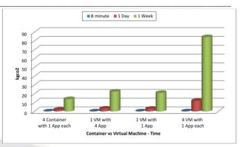
Figure 7. Comparision between Container vs VM for carbon emisison in time intervals.
