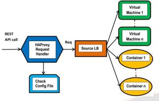
Figure 2. HAProxy Work Flow Design
