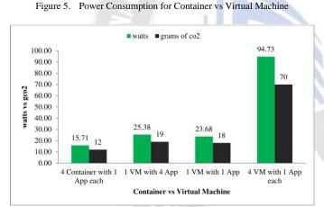
Figure 6. Average Power Consumption vs Carbon Emisison
