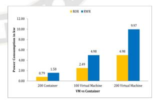
Figure 8. Average Power Consumpton in kw for ROR and RWR
