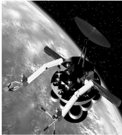
Figure 16. Multiple robotic arms capturing method ATLAS [74]
