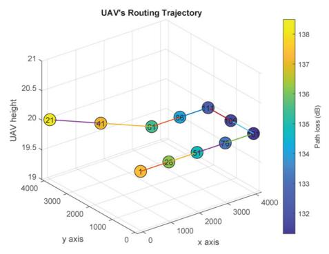
Figure 3.19: UAV's trajectory design over the path loss map using Algorithm 1 (Scenario 1) [4]
