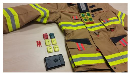
Figure 3.12: Sensors in the suit of the firefighters [44]
