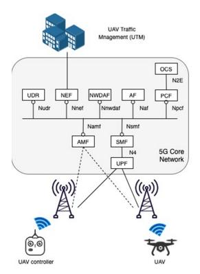
Figure 2.8: The UAV reference model in 5G [22]
