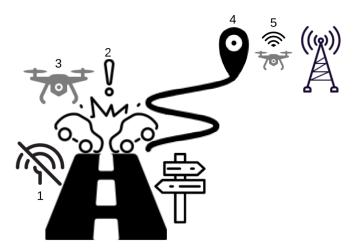
Figure 3.14: The UAV conveys emergency messages and sends them to the closest available network access point [4]
