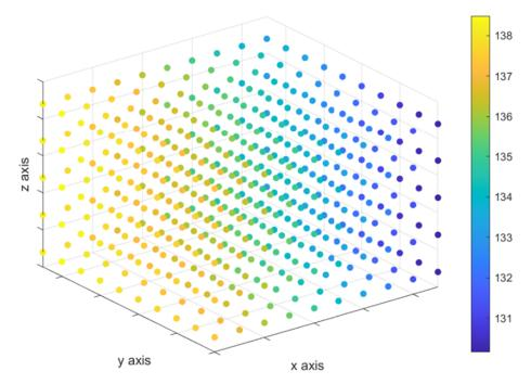
Figure 3.16: Colored path loss map indicating the path loss values (in dB) associated with each point [4]
