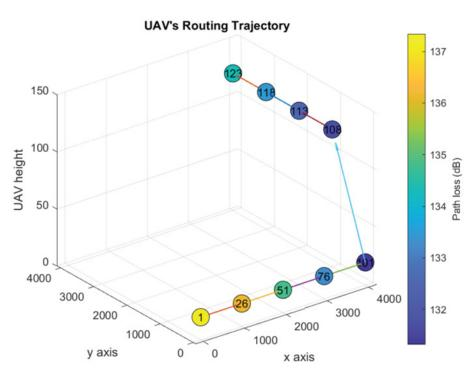
Figure 3.20: UAV's trajectory design over the path loss map using Algorithm 1 (Scenario 2) [4]
