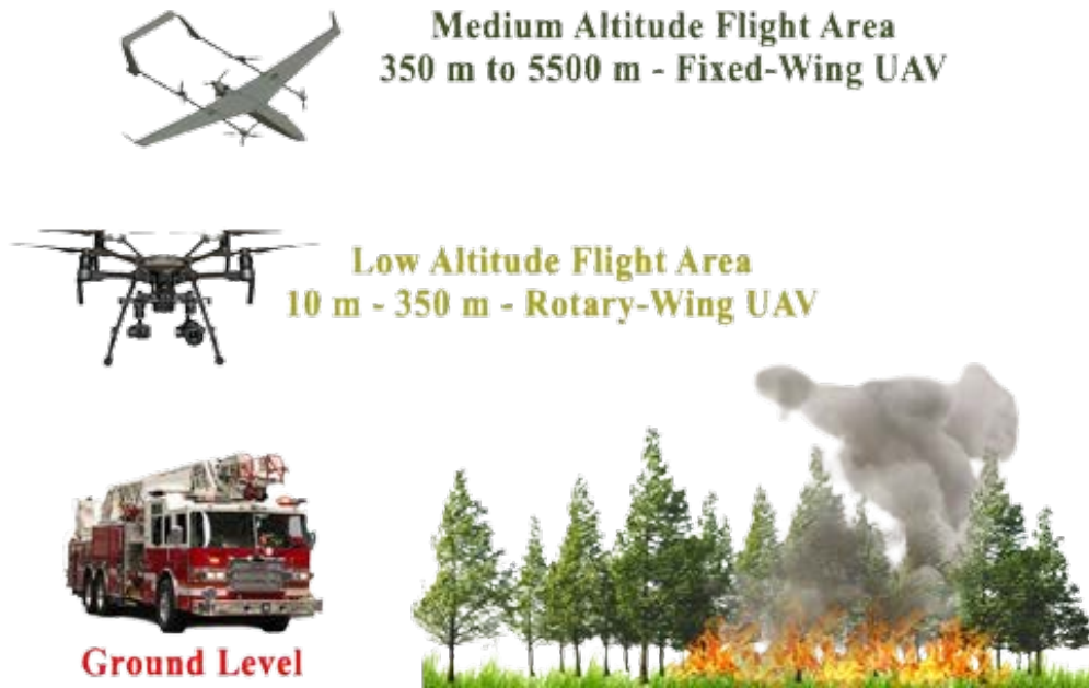
Figure 2.4: Fire Detection with the use of 2 UAV's
