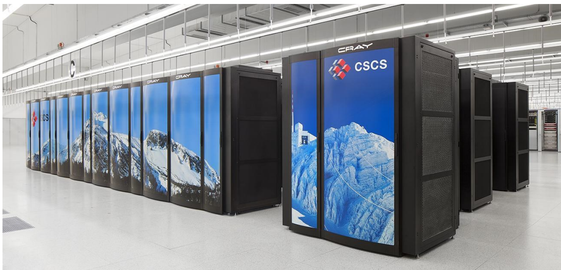
Figure 5: PIZ DAINT CRAY XC50, XEON E5-2690V3 12C 2.6GHZ, ARIES INTERCONNECT, NVIDIA TESLA P100 located in Swiss National Supercomputing Center
