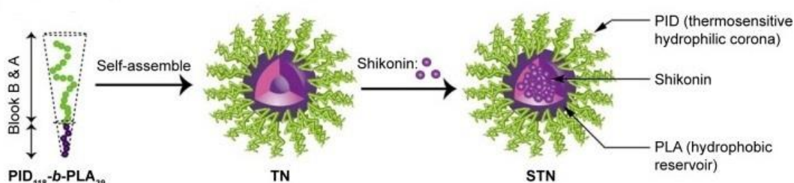
Figure 9: The assembly process of the shikonin-loaded thermoresponsive nanomicelle (STN) with PNIPAM-co-DMAAm (PID) as the hydrophilic corona and polylactic acid (PLA) as the hydrophobic reservoir (Source: Yonghua Su et al., Successful in vivo hyperthermal therapy toward breast cancer by Chinese medicine shikonin-loaded thermosensitive micelle , Int J Nanomedicine 2017; 12:4019-4035).
