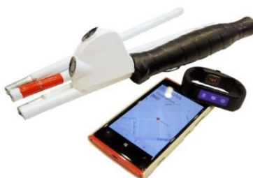
Figure 33: The BAWA Cane with a mobile and the wearable device (wrist band)
