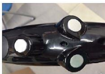
Figure 8: The three ultrasonic sensors of the cane
