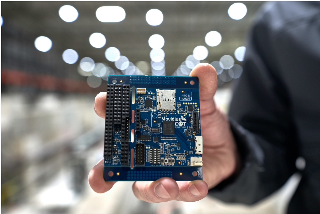
Figure 3.1: Intel's Myriad 2 Vision Processing Unit during radiation testing for space at CERN [3]
