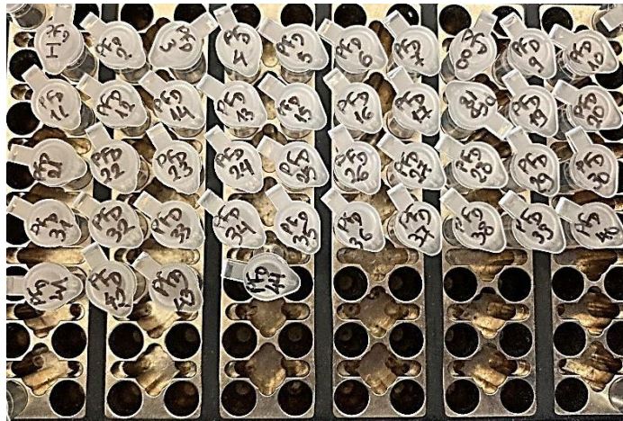
Image 8. cDNA samples ready to be incubated at 42 degrees Celsius for one hour.
