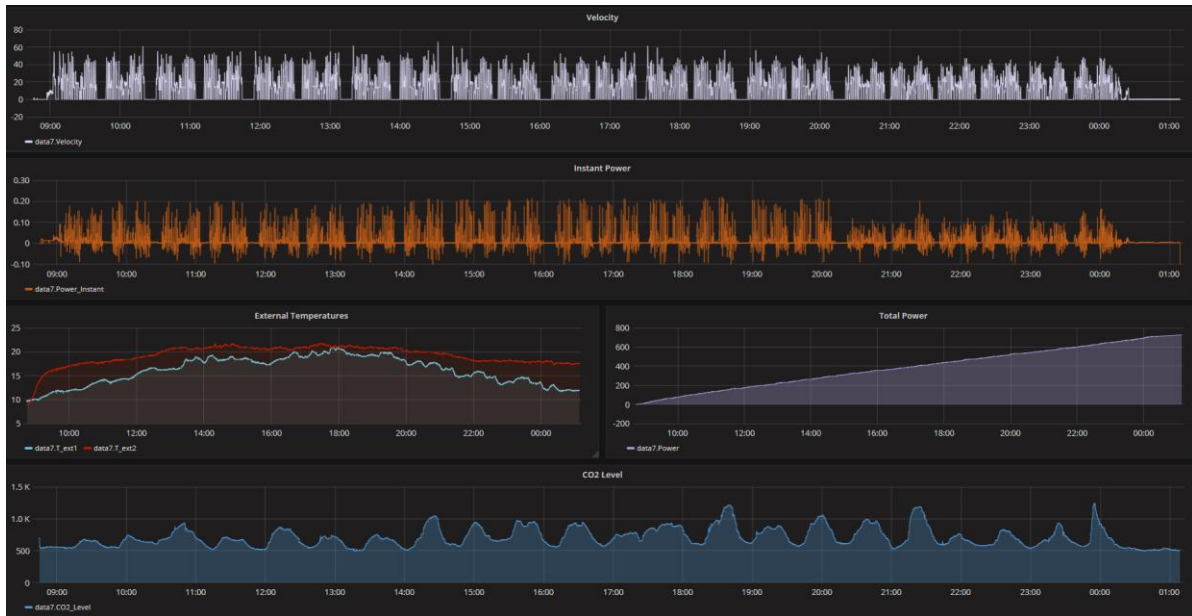
Figure 43: Plots for Velocity, Instant Power, External Temperature 1, External Temperature 2, Total Power, and CO2 Level for the duration of a single day.
