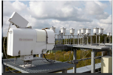
Figure 3.2 Map with the location of MOL-RAO pinpointed (left), photometric devices installed and functioning on a tracker at MOL-RAO (upper right) and a microwave radiometer along with pyranometers at MOL-RAO (lower right)
