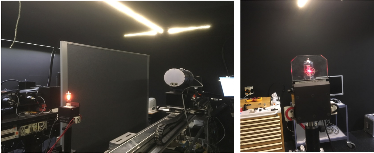
Figure 3.10 PSR calibration at PMOD/WRC laboratory. (Left) Calibration reference lamp used for PSR calibrations in PMOD/WRC laboratory (Right).
