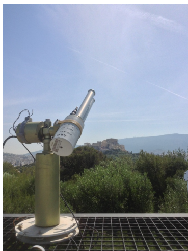
Figure 3.8 Cimel sun photometer installed and running at NOAA's Actinometric station.
