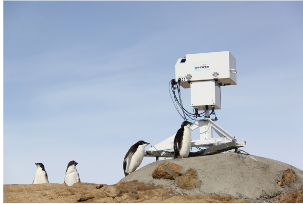
Figure 3.12 A Brewer spectroradiometer installed in Antarctica.
