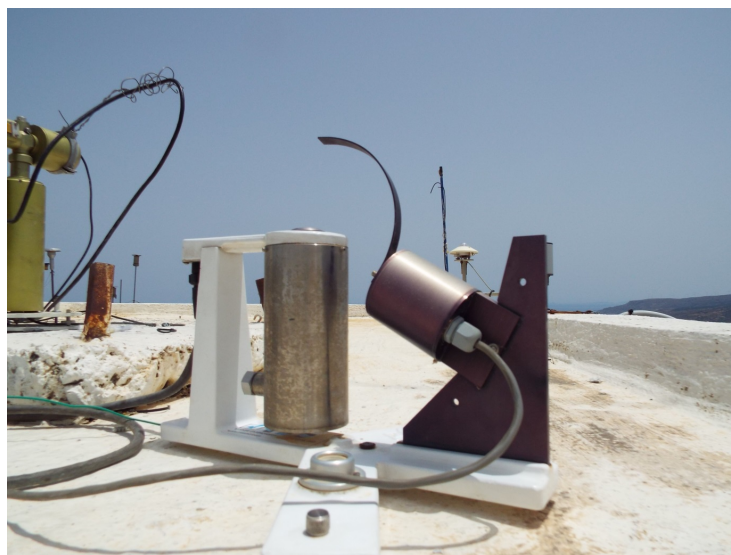
Figure 3.3 UVMFR installed and functioning at FINOKALIA, Greece.
