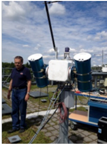
Figure 5.1. PSR#004 and PSR#006 installed on a sun tracking device at MOL-RAO,
