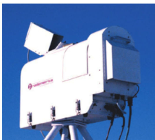
Figure 3.14 MWP, MP-3000A installed at MOL-RAO
