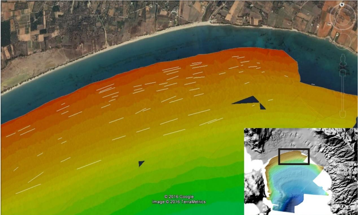
Fig.4.5: Swath bathymetry map of the northern shallow part of the Bay of Vatika. The white bars show the width of the paleo-channels as measured on the 3.5 kHz profiles.
