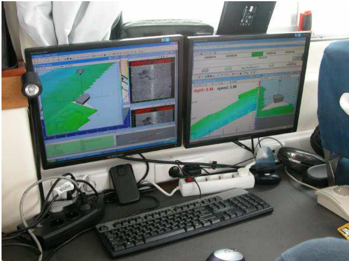
Fig.2.2: The monitors of the deck unit of the RESON Sea Bat 7125 multibeam system onboard RV Alkyon.
