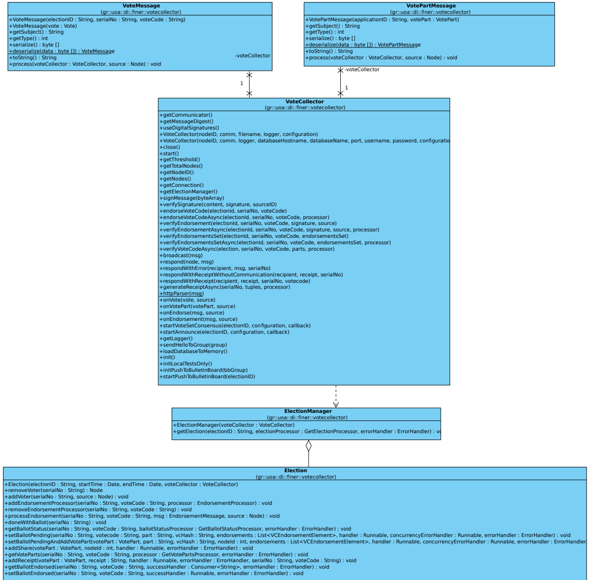
Figure 5.2: A UML Class Diagram of the voting protocol related classes of the Vote Collector implementation.
