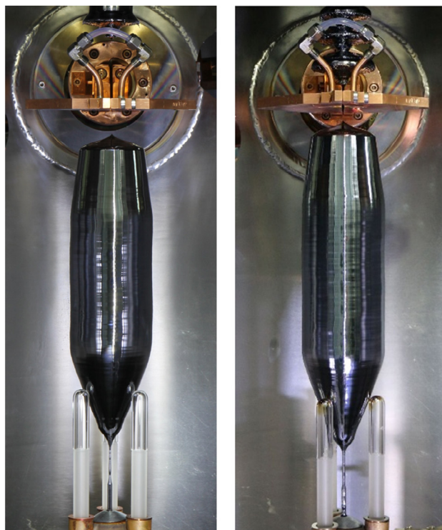
Figure 8. The final FZ mono-crystals of the kg-2 project (charge 23 (left) and 24 (right)), grown in 2015 and in 2016, respectively. The crystals have a \langle 100 \rangle crystallographic orientation.
