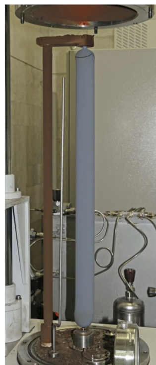
Figure 6. Polycrystalline silicon rod of charge 23 in the deposition apparatus (length of the rod about 85 cm).
