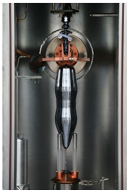
Figure 3. Final single crystal of the IAC Project, grown in 2007 (charge 10) [12]. John Wiley & Sons. [Copyright © 2010 WILEY-VCH Verlag]
