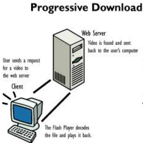
Figure 1.1: Progressive download architecture
