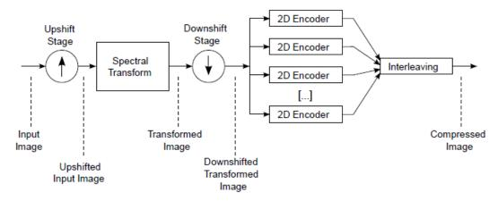
Figure 2.1: Block Diagram of the Compressor for 3D Images
