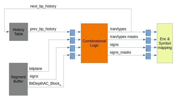
Figure 3.4: Block Diagram of BSMS design with pipeline (1/2)
