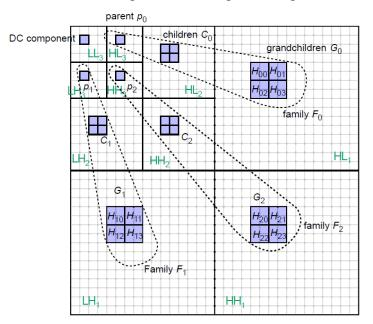
Figure 2.3: Schematic of Wavelet-Transformed Image
