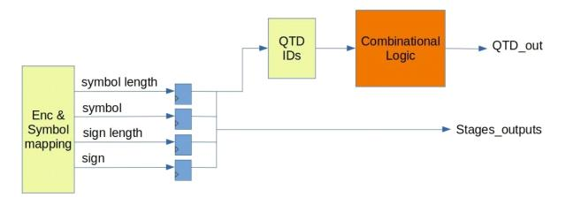
Figure 3.5: Block Diagram of BSMS design with pipeline (2/2)
