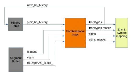
Figure 3.2: Block Diagram of BSMS design without pipeline (1/2)
