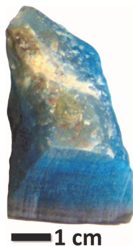
Figure 1. Blue Cu-bearing smithsonite sample from Lavrion historical mines (courtesy of the Mineralogy and Geology Museum of the NTUA, Greece).
