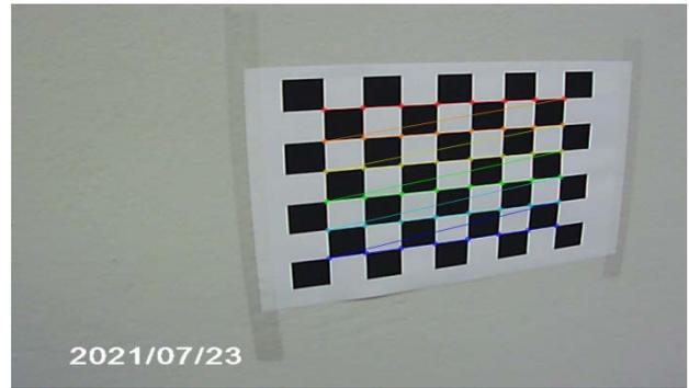
**Image 16: Result of undistorted image with checker board corners detected**
