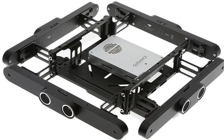
**Image 1: DJI's Guidance Obstacle Avoidance System [42]**
