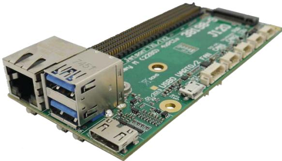
**Image 12: Auvideo J120A-IMU/MCU carrier for Jetson TX1/TX2 [46]**
