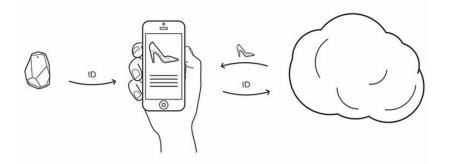
Figure 39: Beacon, BLE and cloud communication
