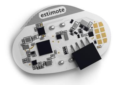
Figure 38: The "inside" of an Estimote location beacon
