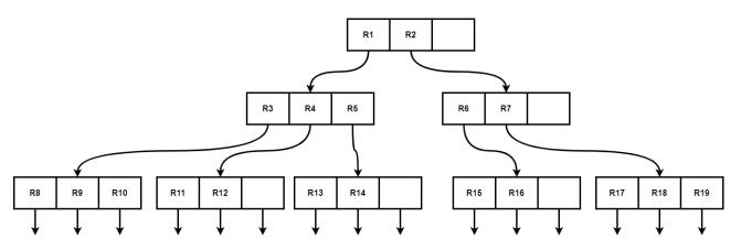
Figure 20. The R-Tree data structure.
