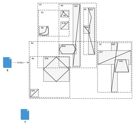
Figure 22. R-Tree: Indexing the source dataset.
