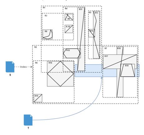
Figure 23. R-Tree: Find the nodes the target geometry resides in.
