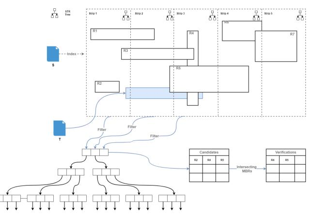
Figure 18. Strip STR Sweep: Verify the candidate geometries that have intersecting MBRs.
