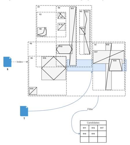
Figure 24. R-Tree: Each geometry belonging to the selected nodes is a candidate.
