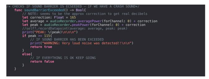
Image 5.6: Function which detects abnormally high noise volume inside the car.
