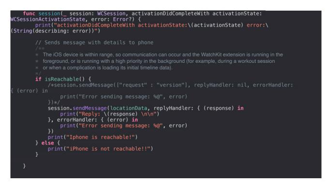
Image 5.7: Function which establishes a connection between the user's iPhone and Apple Watch.
