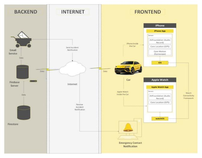
Figure 3.0: Application's Architecture (Backend and Frontend).
