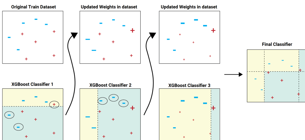
Figure 18: XGBoost classifier training process. Each sub-classifier learns from previous errors and re-adjusts the weights. This process continues until we have a combined final classifier that predicts all the data points correctly
