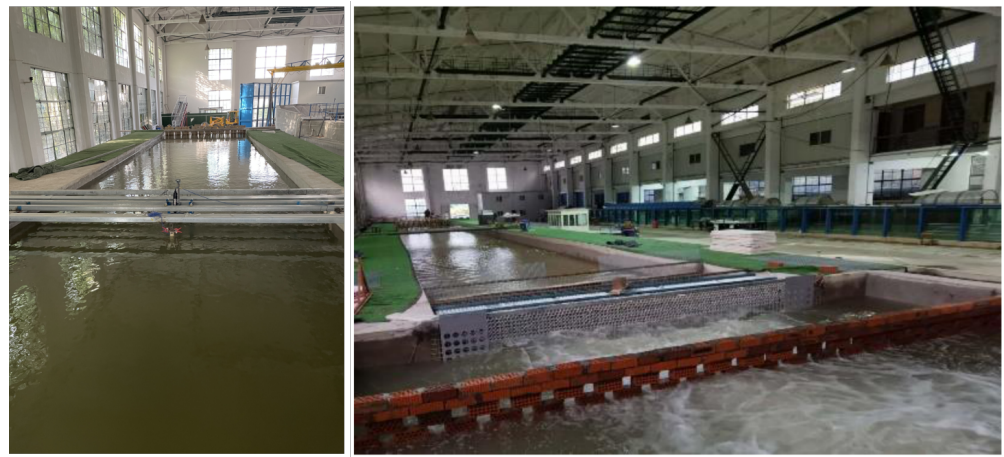
Figure 1. Experimental setup at the circulating flow flume. The left picture shows the movable platform on which the Nortek Vectrino Profiler is positioned. The right picture shows the porous walls at the inlet of the flume.
