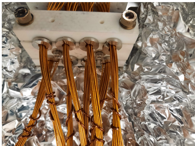
Fig. 5. Close up view of the MACOR strain reliefs mounted to the cable harnesses. Kapton cables are separated into bundles of 8–10 wires to be fed through strain relief. Additional stainless steel funnels were placed within strain reliefs to reduce wire stress.
