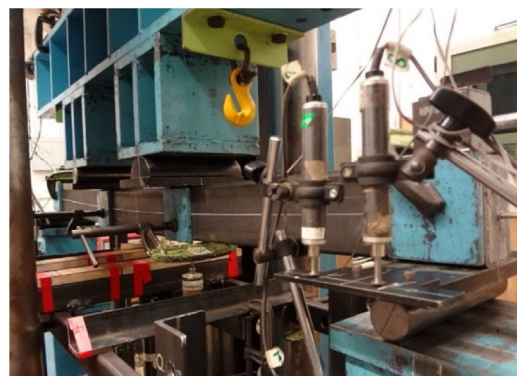
Fig. 5. Four-point bending test setup (a) Schematic view (b) Actual beam test.
