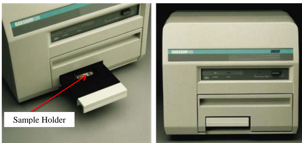
Figure 3-1. TSL experimental setup (Harshaw QS 3500)
