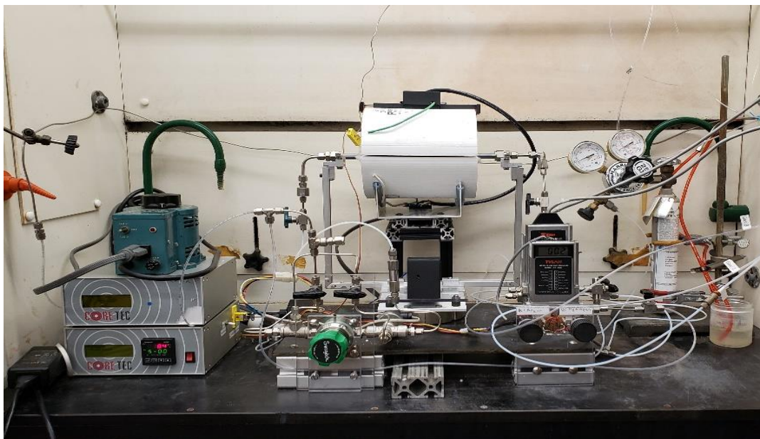
Figure 7: Plug-flow reactor. The catalyst is contained in a stainless-steel tube, which is subjected to heating and the flow of gases. The flow of gases through the reactor is controlled by two mass flow controllers, which are calibrated for nitrogen. Finally, the back pressure regulator (BPR) maintains a certain pressure throughout the system.
