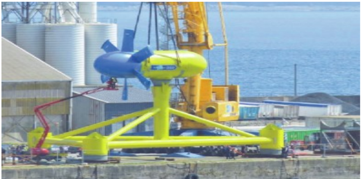
Figure 3. Sabella D10 tidal turbine dockside in Brest before installation. Source (energylivenews.com)
