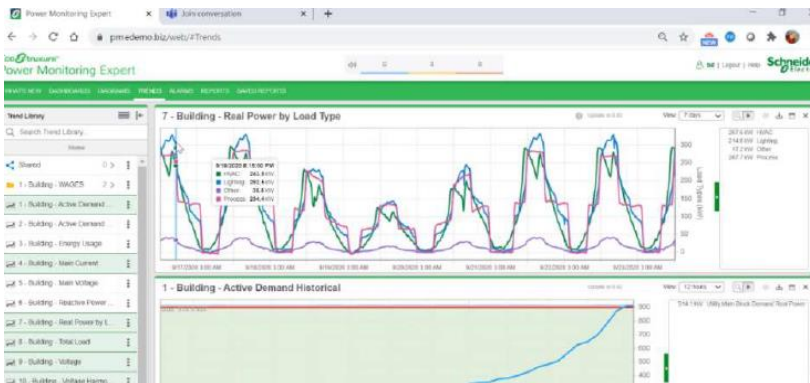
(c) Analysis of different loads connected to the station with power
