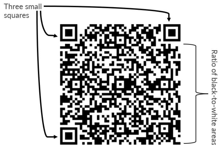
Figure 3: QR Codes Anchoring by Squares in the Corner - 360-degree Photo -New Giza University Project
