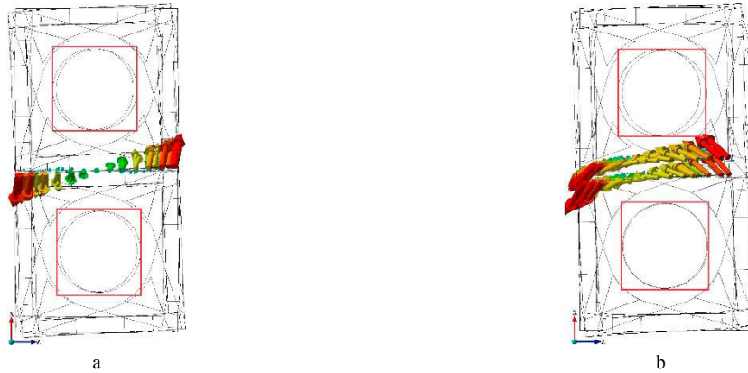
Fig. 3. Asymmetric deformation behavior in the system of two cells created by (a) “joining” and (b) “overlapping” methods.
