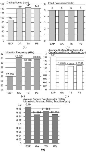
Figure 4. The Most Efficient Optimized Input and Outputs
