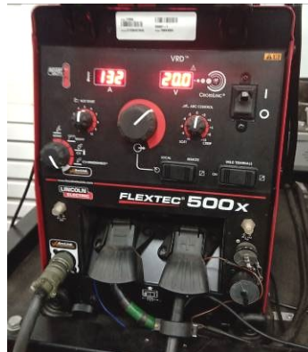
Fig. 2. PLEXTEC® 500x welding machine and welding process parameters
