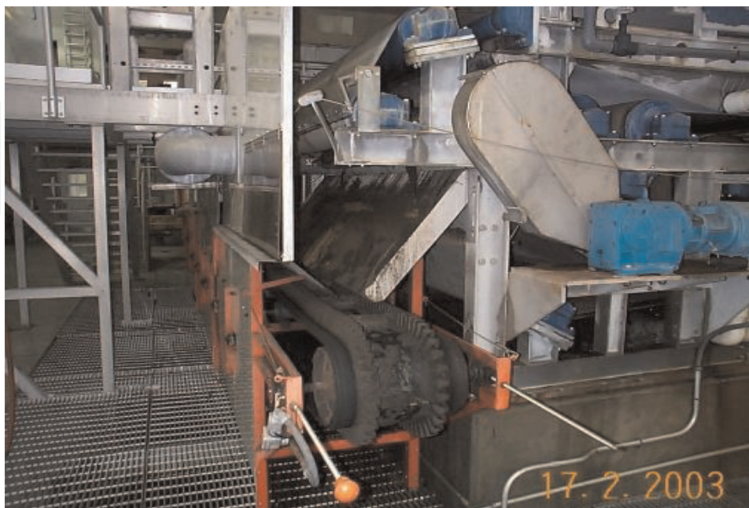
Figure 8. Belt press used to treat sewage solids (with TRIO 3 permitted authorization).
