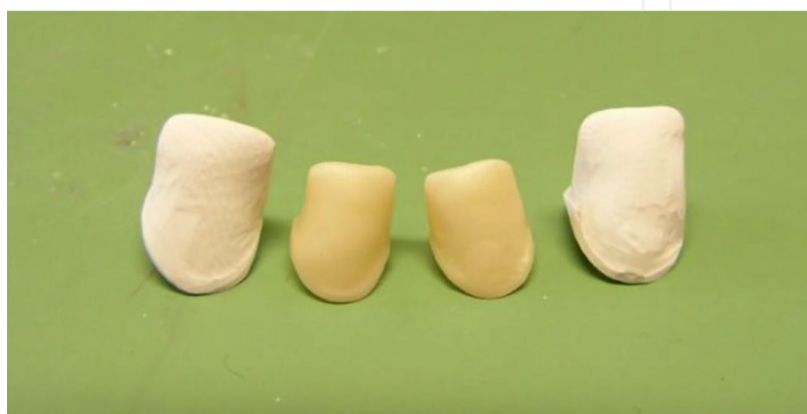
Figure 10. Zirconia blocks before and after staining and sintering. The shrinkage is easily observed.
