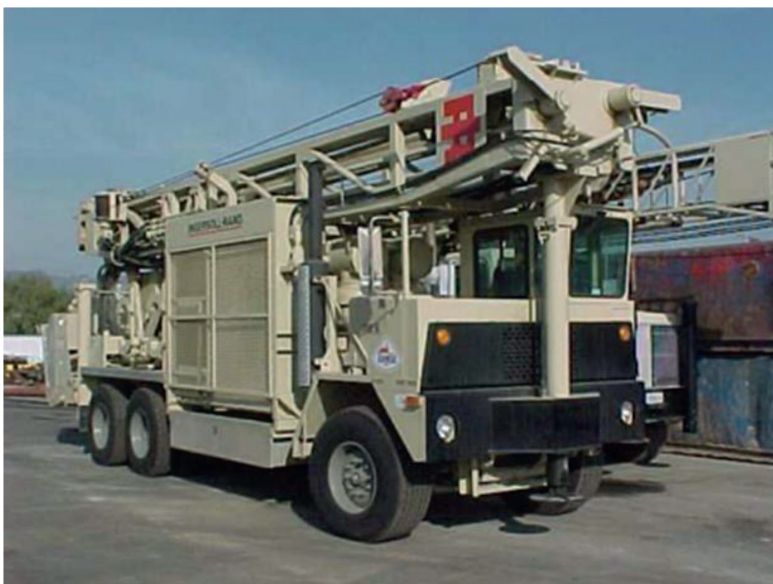
Figure 7. An air rotary drilling rig in transport configuration [31].
