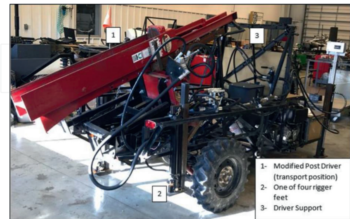
Figure 17. Well-Driver PUP vehicle in transport configuration with the hydraulic driving ram collapsed into holding cradle [44].
