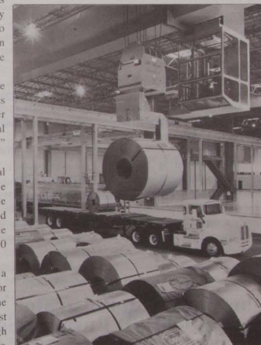
Operator of 30-ton computerized crane hoists 38,000 pound roll of steel and prepares to load it on awaiting truck for delivery at a new $12 million transloading facility for Budway Truck in Fontana, CA. Built by Oltmans Construction Co. of Whittier, CA, the 120,000-sq.-ft. plant features two computerized cranes, a concrete floor thick enough to handle major airliners, and can accommodate 60 rail cars at a time.
