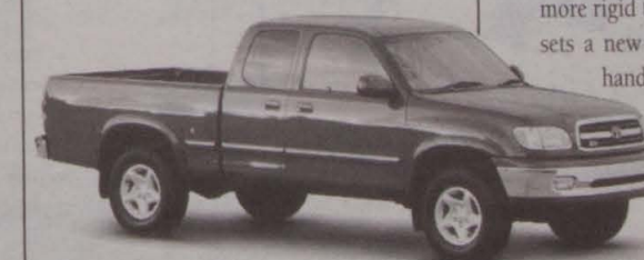
The Tundra's V8 delivers 245 horsepower and 315 pounds-feet of torque and still achieves L.E.V. (low emissions vehicle) emissions classification.
