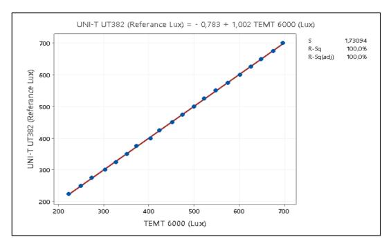
Figure 14. Regression equation and coefficient based on UNI-T UT382 vs. TEMT6000 the measurement.
