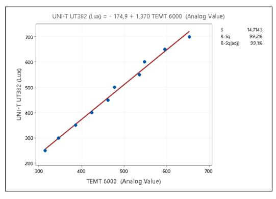
Figure 11. Regression equation and coefficient based on UNI-T UT382 vs. TEMT6000 for the calibration
