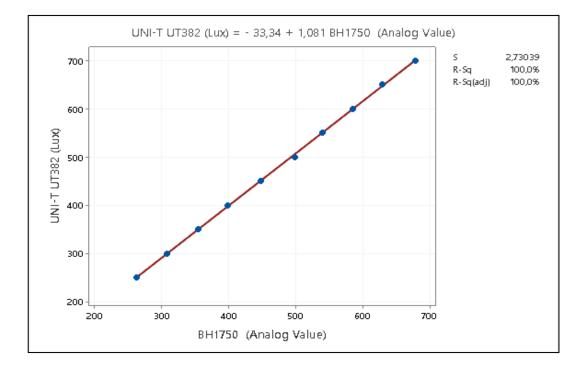
Figure 10. Regression equation and coefficient based on UNI-T UT382 vs.BH1750 for the calibration
