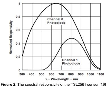
Features of the TSL2561 sensor can be ordered as precisely brightness measurements under different lighting conditions, work on -30 to 80 °C temperature scale, 0.1 to 40,000 lux in a dynamic scale measurement, work at 2.7-3.6V voltage scale and I2C interface [19].
